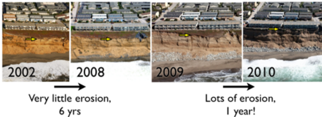
Figure 5. Changes over time in coastal bluffs in Pacifica California. They go for many years without much erosion and then erode more than a dozen feet in a single year. The yellow triangle shows the migration of the cliff top from year to year at a single position. By 2010, the cliff is located directly beside the apartment building. (California Coastal Records Project 2013)
